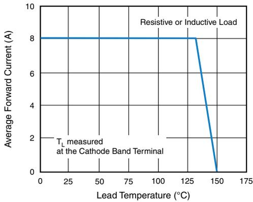
Fig. 1 - Maximum Forward Current Derating Curve
