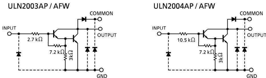
(Note) : The input and output parasitic diodes cannot be used as clamp diodes.
