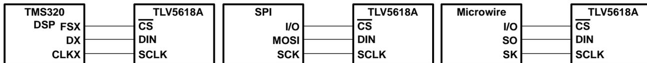
**Figure 12. Three-Wire Interface**
