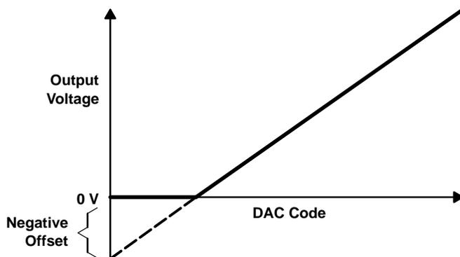
Figure 8. Effect of Negative Offset (Single Power Supply)
