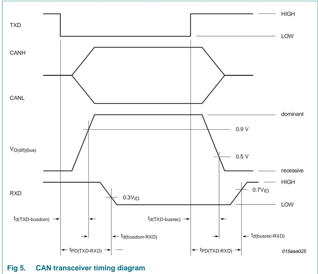
Fig 5. CAN transceiver timing diagram
