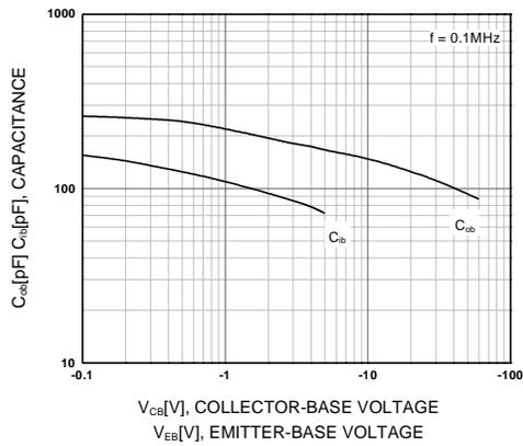
Figure 3. Output and Input Capacitance
