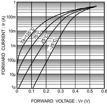
Fig. 1 Forward characteristics
