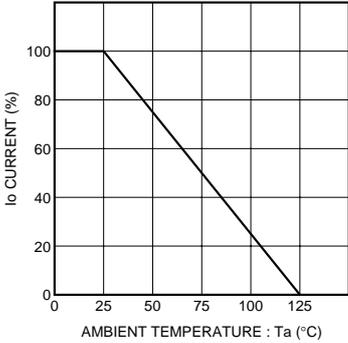
Fig. 4 Derating curve (mounting on glass epoxy PCBs)
