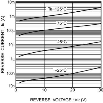
Fig. 2 Reverse characteristics
