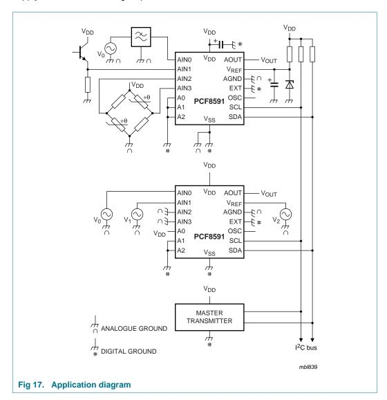
8-bit A/D and D/A converter
