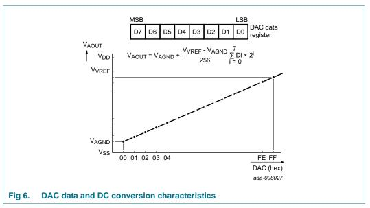
8-bit A/D and D/A converter
