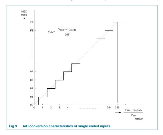
8-bit A/D and D/A converter
