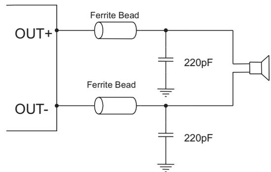
Figure 2: Ferrite Bead Filter to reduce EMI
