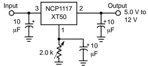
Figure 29. Adjusting Output of Fixed Voltage Regulators
