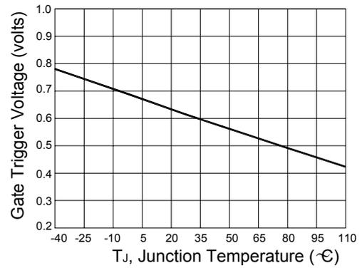
**Figure 2. Typical Gate Trigger Voltage Versus Junction Temperature**
