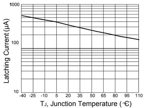
**Figure 4. Typical Latching Current Versus Junction Temperature**
