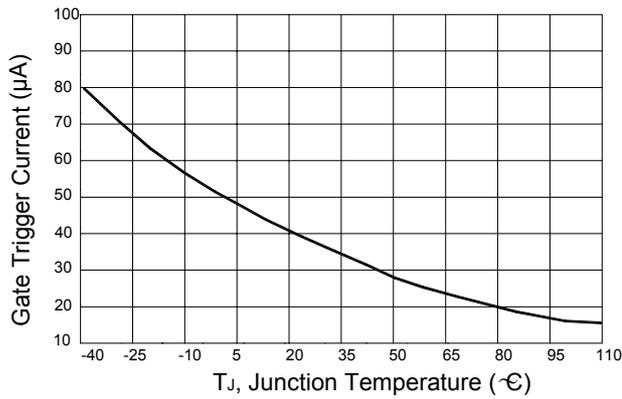
**Figure 1. Typical Gate Trigger Current Versus Junction Temperature**
