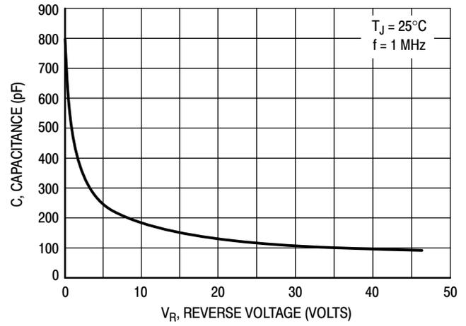
Figure 8. Typical Capacitance
