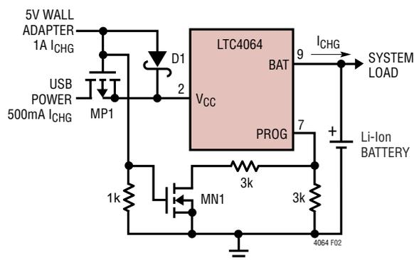
Figure 2. Combining Wall Adapter and USB Power
