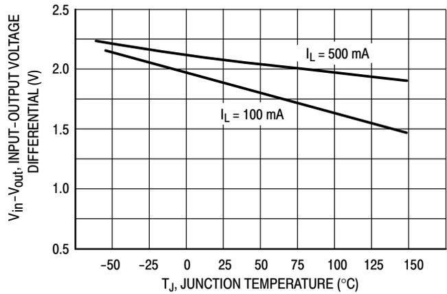
Figure 10. Dropout Voltage
