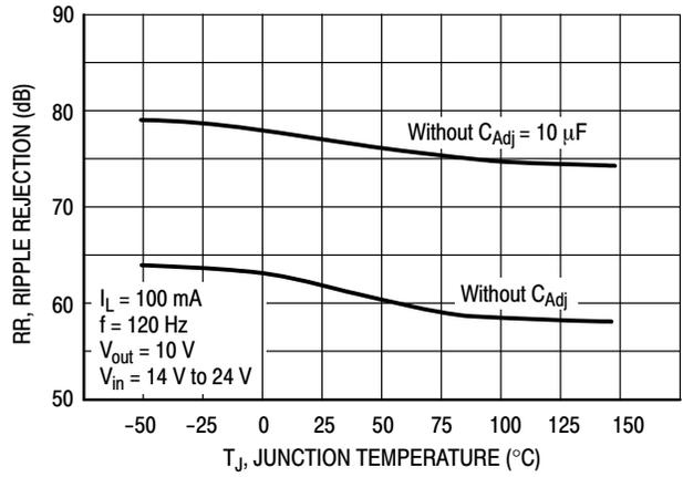
Figure 8. Ripple Rejection
