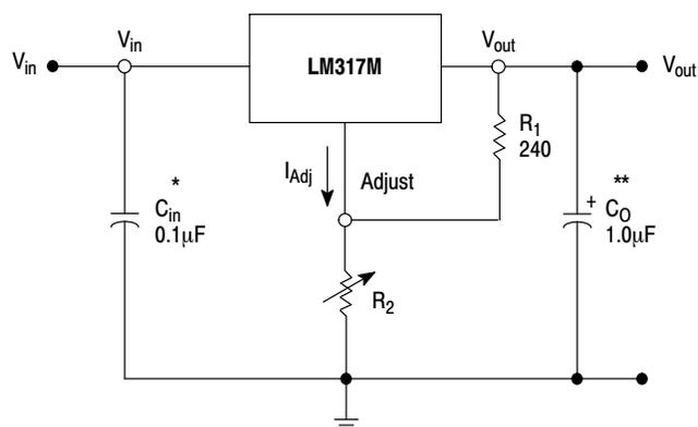
\* =  $C_{in}$  is required if regulator is located an appreciable distance from power supply filter.
