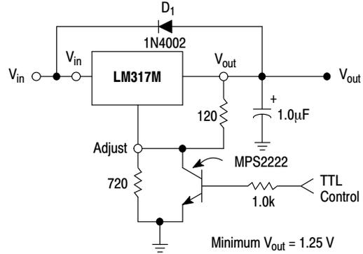
$D_1$  protects the device during an input short circuit.
