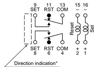
Diagram shows the "reset" position when terminals 2 and 15 are energized. Energize terminals 1 and 16 to transfer contacts.
