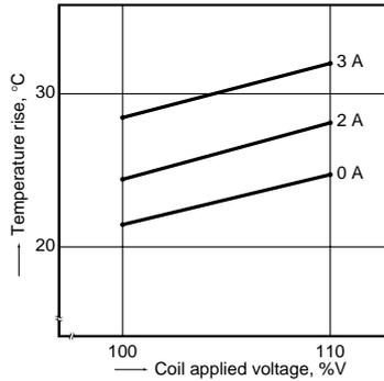
**2-(2) Coil temperature rise 2 coil latching**
