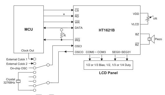
Note: The connection of  $\overline{IRQ}$  and  $\overline{RD}$  pin can be selected depending on the requirement of the MCU.
