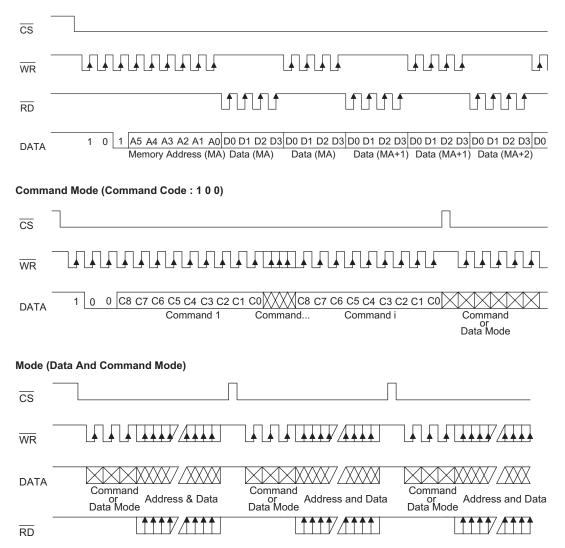
Note: It is recommended that the host controller should read in the data from the DATA line between the rising edge of the  $\overline{\text{RD}}$  line and the falling edge of the next  $\overline{\text{RD}}$  line.
