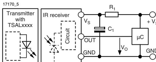
$R_1$  and  $C_1$  are recommended for protection against EOS. Components should be in the range of  $33 \Omega < R_1 < 1 \text{ k}\Omega$ ,  $C_1 > 0.1 \mu\text{F}$ .
