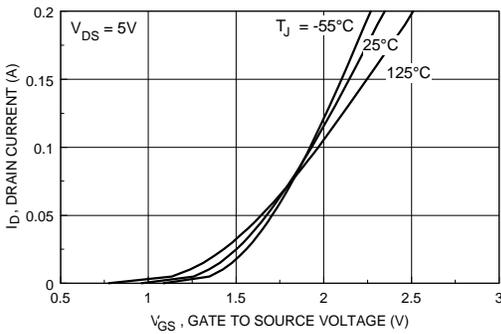
Figure 5. Transfer Characteristics.
