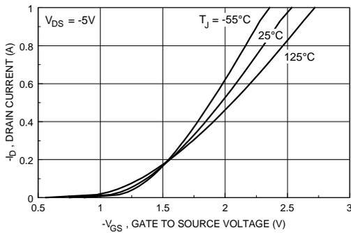
Figure 15. Transfer Characteristics.
