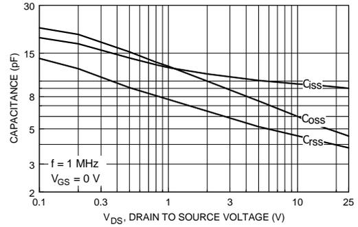
Figure 8. Capacitance Characteristics.
