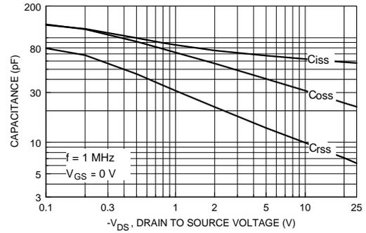
Figure 18. Capacitance Characteristics.
