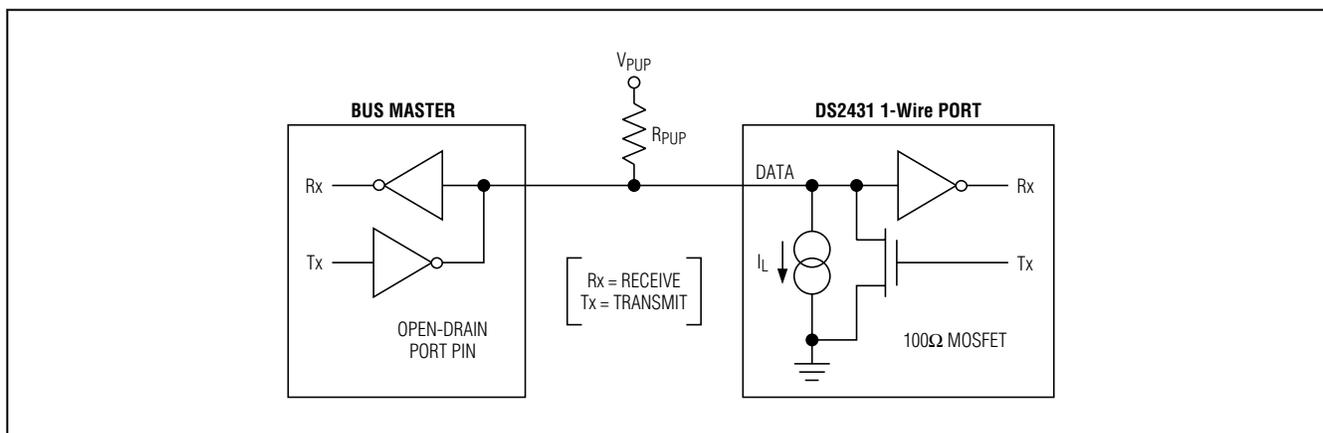
Figure 8. Hardware Configuration
