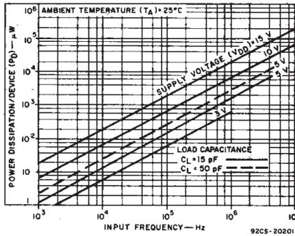
Fig. 8 — Typical power dissipation vs. frequency.
