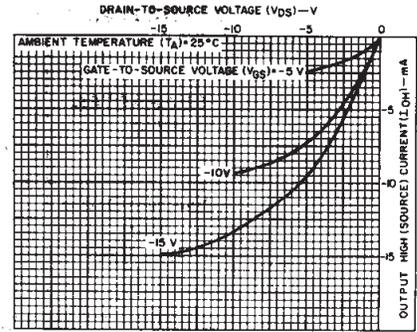
Fig. 5 — Minimum output high (source) current characteristics.
