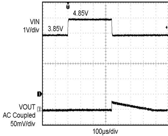
Figure 18. Line Transient Response (3.85 V to 4.85 V)
