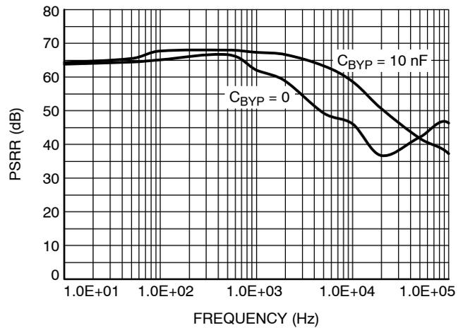
Figure 13. PSRR vs. Frequency (10 mA Load)
