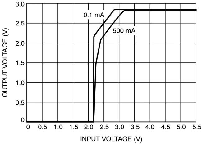
Figure 3. Dropout Characteristics
