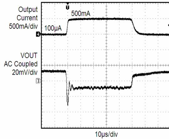
Figure 19. Load Transient Response (0.1 mA to 500 mA)
