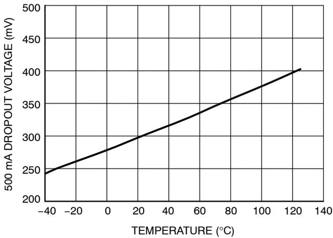
Figure 10. Dropout vs. Temperature (500 mA Load)
