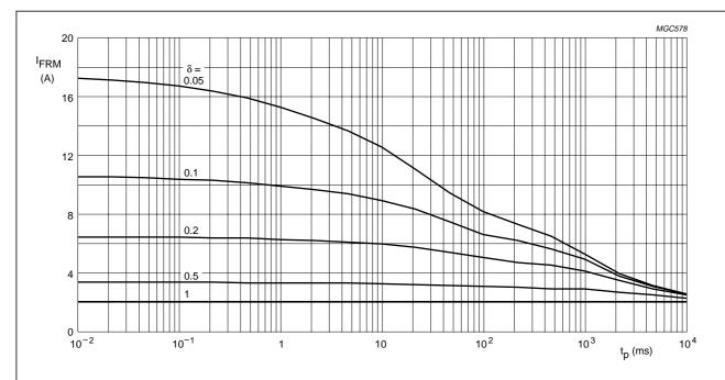
$$\begin{split} T_{tp} = 65 \text{ °C}; & R_{th,j-tp} = 46 \text{ K/W}. \\ V_{RRMmax} & \text{during 1} - \delta; \text{ curves include derating for } T_{j,max} \text{ at } V_{RRM} = 600 \text{ V}. \end{split}$$
