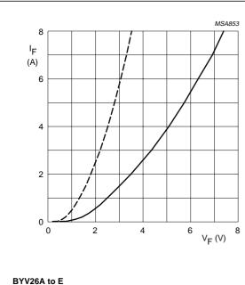
Dotted line:  $T_j = 175 \,^{\circ}C$ . Solid line:  $T_j = 25$  °C.
