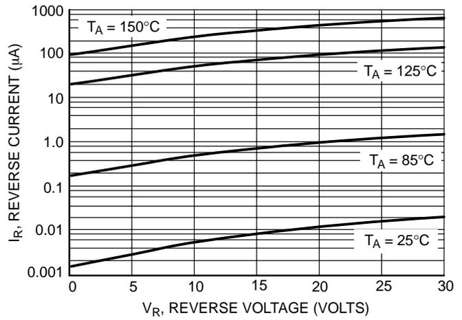
Figure 3. Leakage Current
