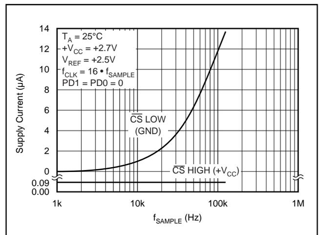
FIGURE 9. Supply Current vs State of  $\overline{CS}$ .
