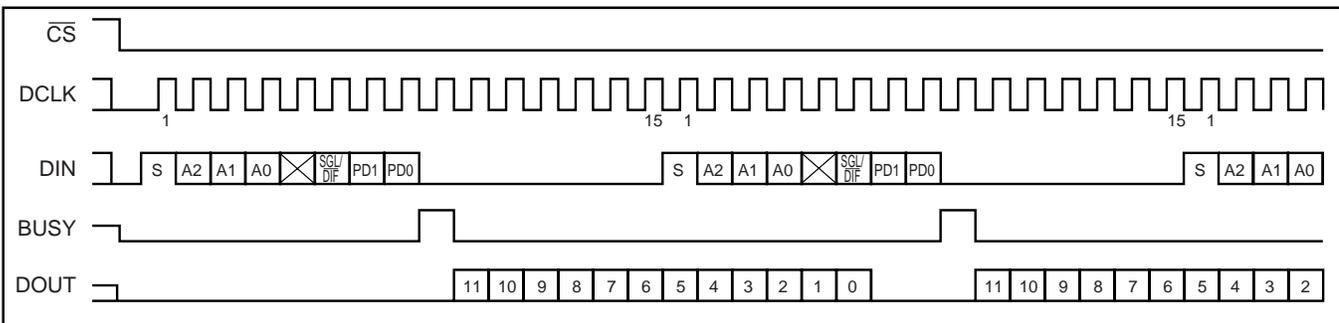
FIGURE 6. Maximum Conversion Rate, 15-Clocks per Conversion.
