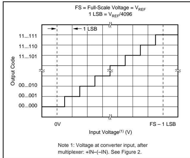
FIGURE 7. Ideal Input Voltages and Output Codes.
