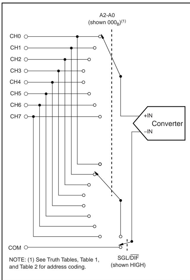
FIGURE 2. Simplified Diagram of the Analog Input.
