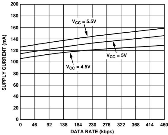
Figure 10. Primary Supply Current vs. Data Rate
