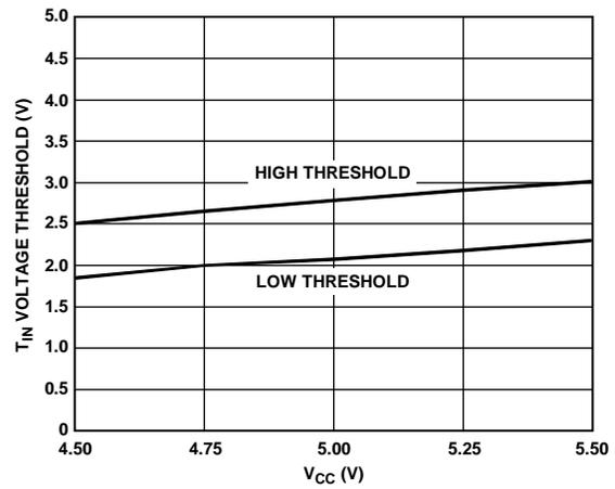
Figure 12. T<sub>m</sub> Voltage Threshold vs. V<sub>CC</sub>
