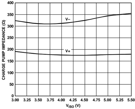
Figure 9. Charge Pump Impedance vs. V<sub>ISO</sub>
