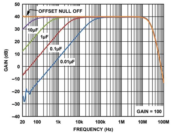
Figure 33. Offset Null Bandwidth vs. Offset Null Capacitor
