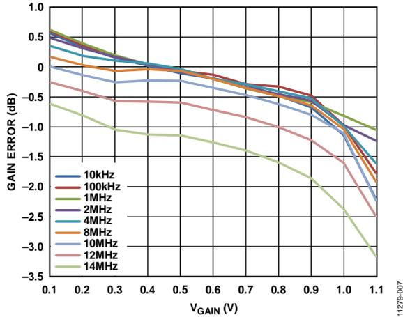
Figure 10. Gain Error vs.  $V_{GAIN}$  over Frequency
