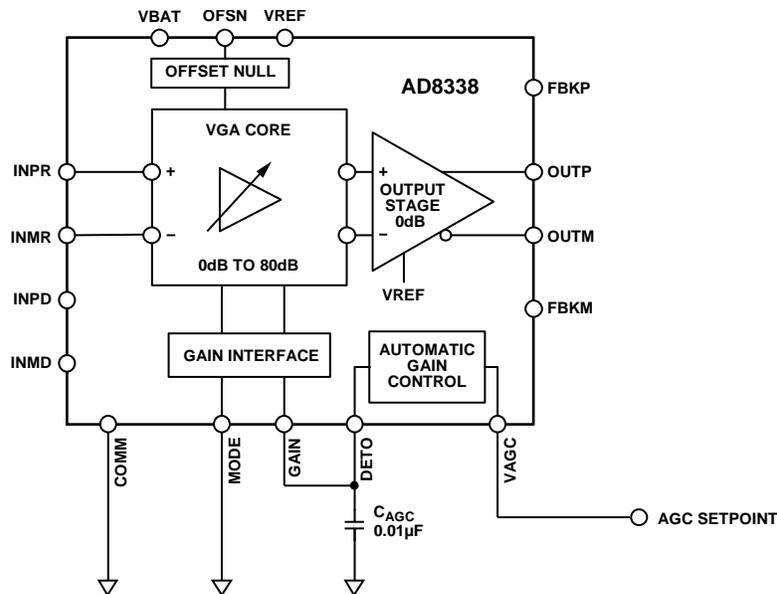
Figure 46. AD8338 Configured as an AGC Amplifier
