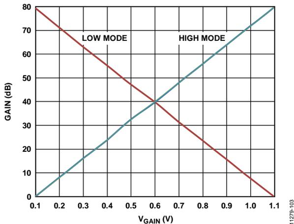
Figure 44. Two Gain Control Modes of the AD8338
