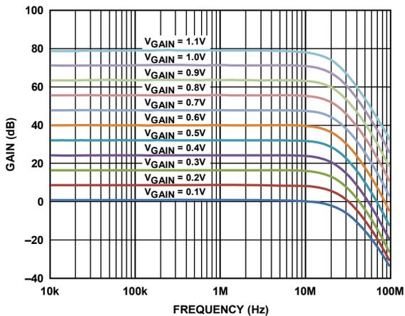
Figure 6. Gain vs. Frequency, 8 dB Steps
