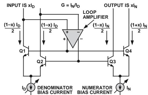
Figure 40. Simplified Diagram of the VGA Core
