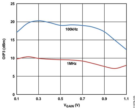
Figure 24. OIP3 vs.  $V_{GAIN}$
