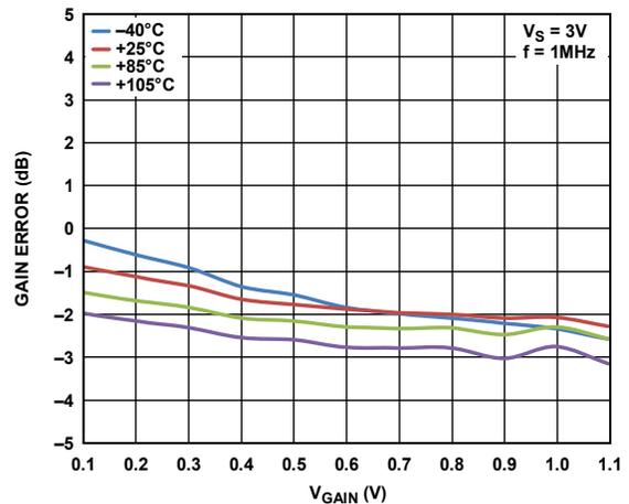
Figure 9. Gain Error vs.  $V_{GAIN}$  over Temperature
