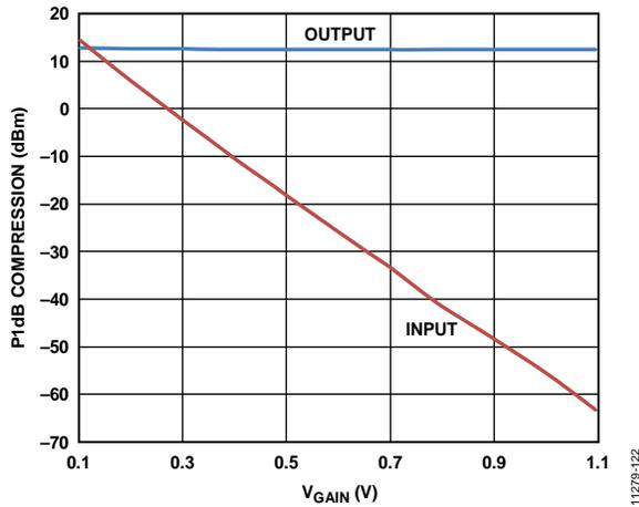
Figure 23. Input and Output 1 dB Compression vs.  $V_{GAIN}$
