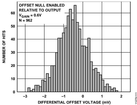
Figure 12. Differential Offset Voltage Histogram
