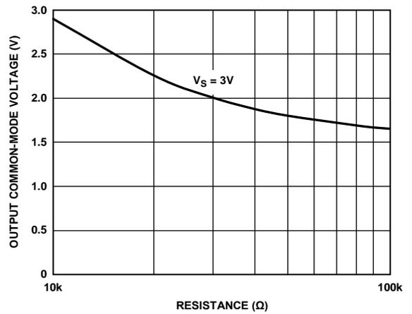
Figure 38. Output Common-Mode Voltage vs.  $R_{CM}$  to COMM
