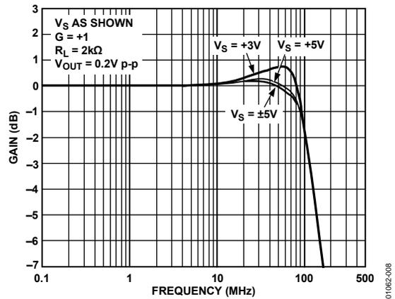
Figure 8. AD8051/AD8052 Gain vs. Frequency vs. Supply
