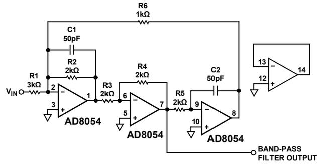
Figure 46. 2 MHz Biquad Band-Pass Filter Using AD8054
