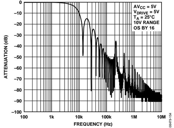
Figure 59. Digital Filter Response for OS 16
