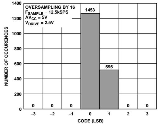
Figure 53. Histogram of Codes—OS  $\times$  16 (Two Codes)
