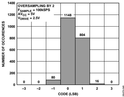
Figure 50. Histogram of Codes—OS  $\times$  2 (Four Codes)
