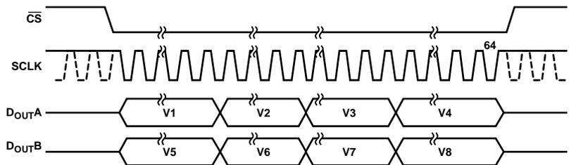
Figure 46. AD7606 Serial Interface with Two  $\text{D}_{\text{OUT}}$  Lines
