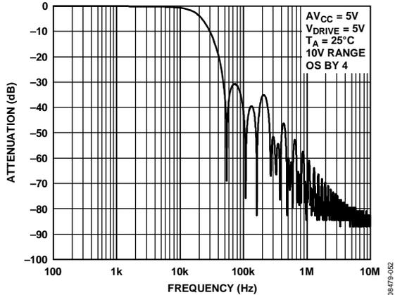
Figure 57. Digital Filter Response for OS 4
