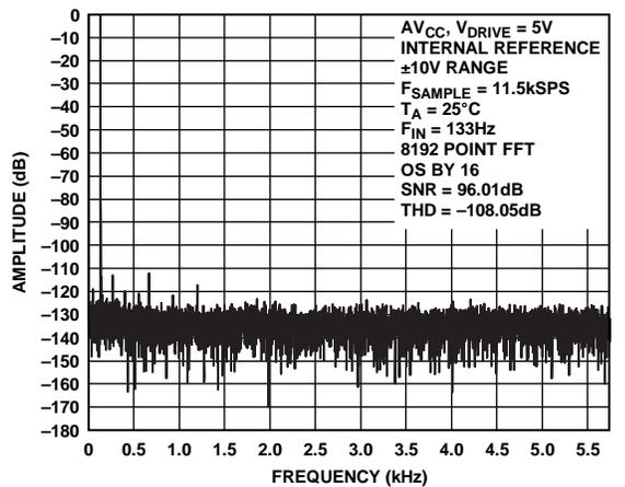
Figure 13. FFT Plot Oversampling By 16, ±10 V Range
