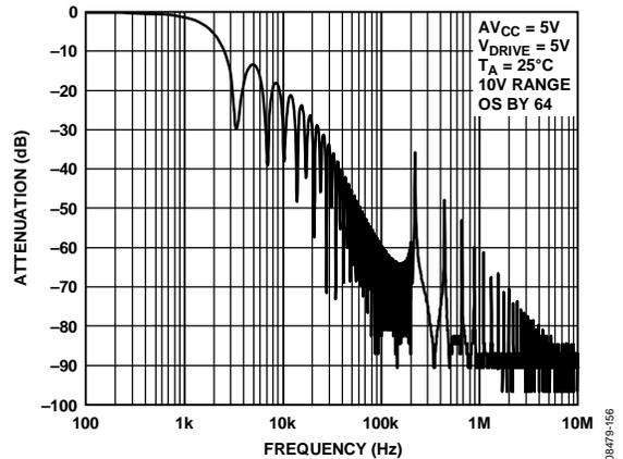
Figure 61. Digital Filter Response for OS 64
