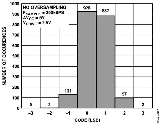
Figure 49. Histogram of Codes—No OS (Six Codes)
