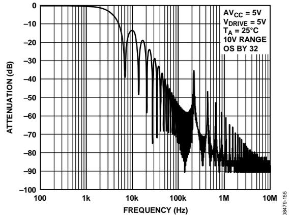
Figure 60. Digital Filter Response for OS 32
