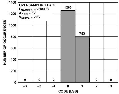
Figure 52. Histogram of Codes—OS  $\times$  8 (Three Codes)
