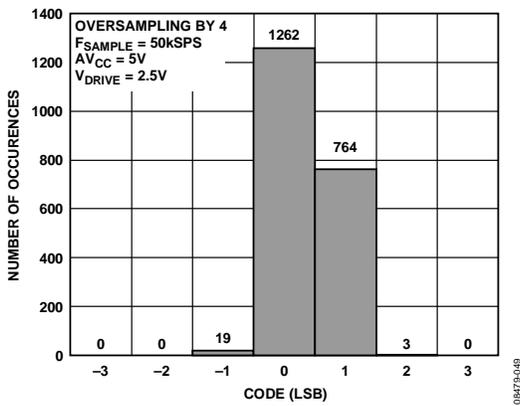
Figure 51. Histogram of Codes—OS  $\times$  4 (Four Codes)
