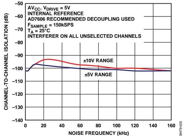
Figure 28. Channel-to-Channel Isolation
