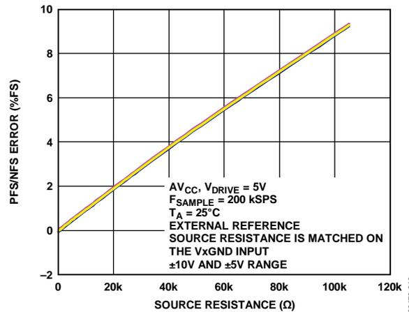
Figure 21. PFS and NFS Error vs. Source Resistance
