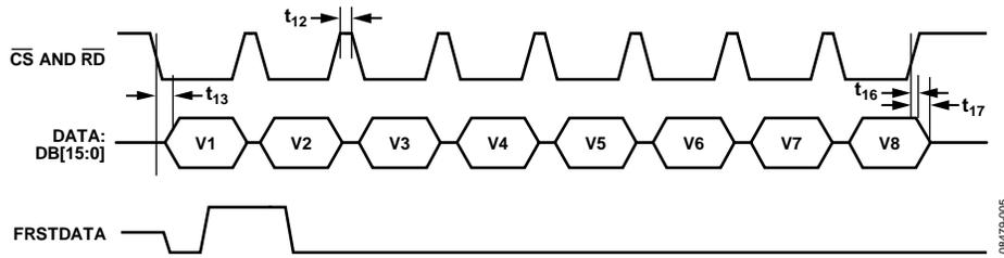
Figure 5.  $\overline{CS}$  and  $\overline{RD}$ , Linked Parallel Mode
