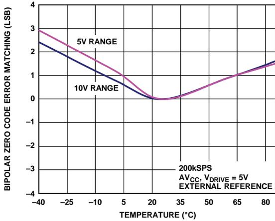
Figure 23. Bipolar Zero Code Error Matching Between Channels
