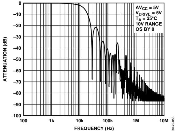
Figure 58. Digital Filter Response for OS 8
