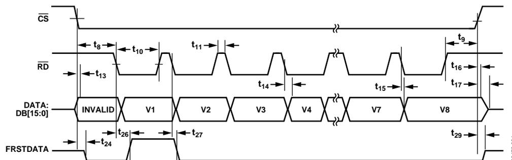
Figure 4. Parallel Mode, Separate CS and RD Pulses
