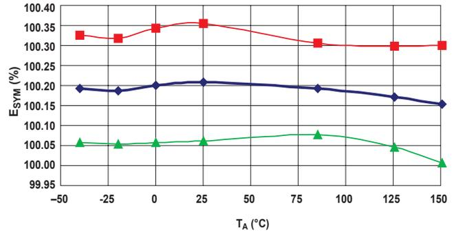
Magnetic Offset Error versus Ambient Temperature
