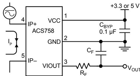
Application 1. The ACS758 outputs an analog signal,  $V_{OUT}$ , that varies linearly with the uni- or bi-directional AC or DC primary sampled current,  $I_p$ , within the range specified.  $C_F$  is for optimal noise management, with values that depend on the application.
