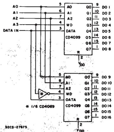
Fig. 14 - 1-of-16 decoder/demultiplexer.
